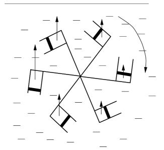
between the neighbouring spokes are equal. The whole setup is under water, and is able to rotate around a horizontal axis going through its center. The volume of the air, due to the heavy pistons, is increased in the cylinders facing down, therefore the buoyancy exerted on these cylinders (on the left side of the figure) is larger than on the other side. As a consequence, the setup will rotate clockwise."
